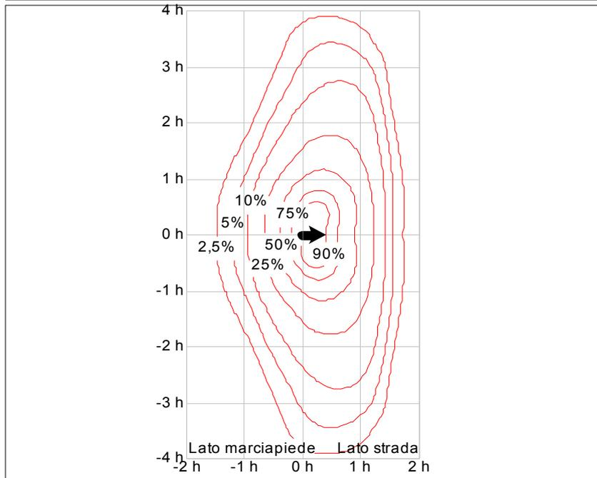
$$E \text{ (lux)} = \frac{E_{\text{max}} \times E\% \times F}{h^2 \times 1000}$$
