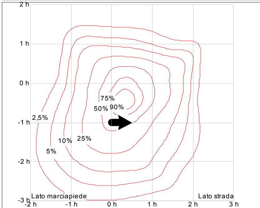
$$E \text{ (lux)} = \frac{E_{max} \times E\% \times F}{h^2 \times 1000}$$
